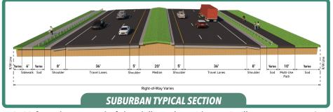
**U.S. 98 from the east end of the Phillips Inlet Bridge to Carillon Avenue** - A 6-lane roadway with curbed shoulders, raised grassed median, 6-foot concrete sidewalk, and a 10-foot multi-use path.
