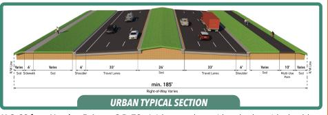
**U.S. 98 from Heather Drive to S.R. 79** - A 6-lane roadway with curbed outside shoulders, raised grassed median, 6-foot concrete sidewalk, and a 10-foot multi-use path.
