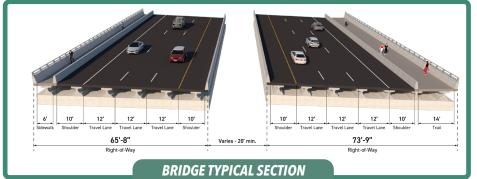
**Phillips Inlet Bridge** - Two new bridge structures with 6 12-foot travel lanes, 10-foot outer shoulders, 6-foot sidewalk, and a 14-foot multi-use path.
