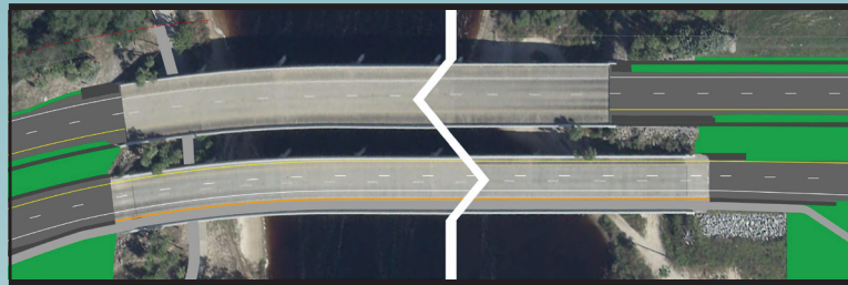
2 Adding concrete barrier wall to continue the sidewalk across the eastbound bridge over Lake Powell
