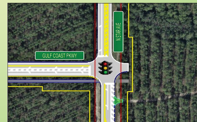
Gulf Coast Parkway and C.R. 2315 (Star Avenue) Proposed Intersection • Beginning project limits • Single turn lanes • Signalized intersection
